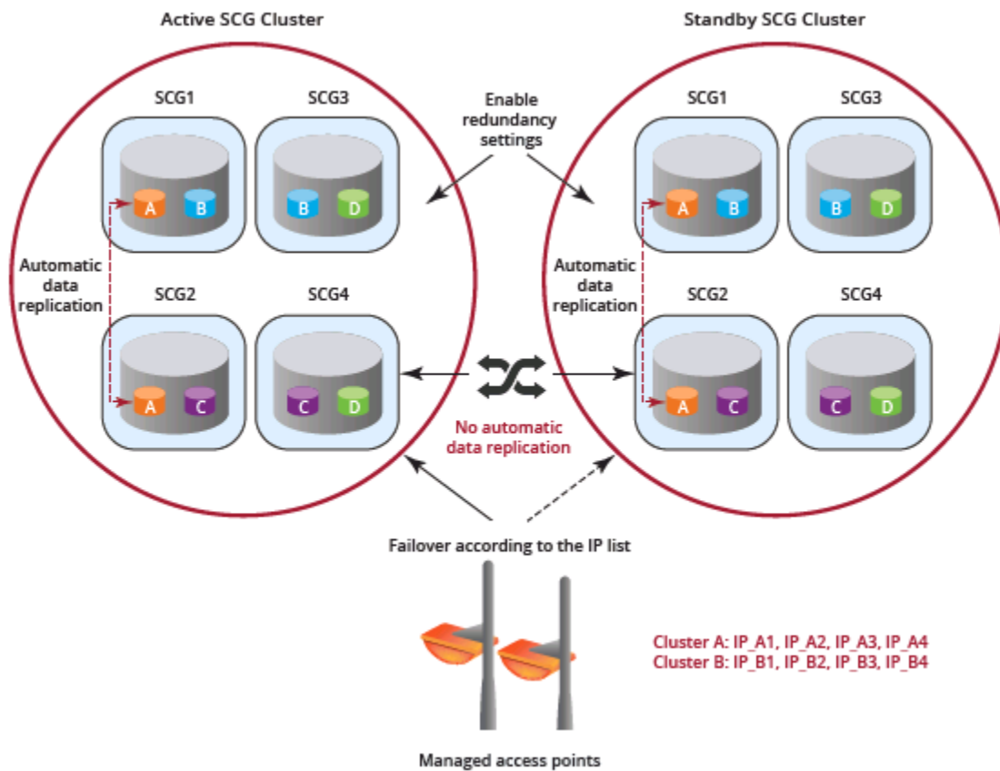
FIGURE 54 Cluster Redundancy for Active-Standby Mode
